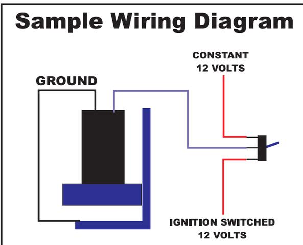
Step 8. Wiring the pump.
