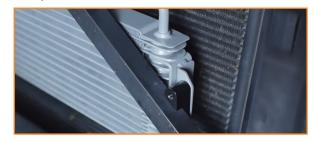
13. Secure the transmission cooler with your mounting hardware. If the cooler is crooked and needs to be adjusted, loosen the button head bolts on the backside of the cooler brackets to adjust its position. (2x brackets, 4x Allen bolts)
