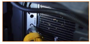
15. Set the line adapters and grommets that are provided in your kit into the recently drilled holes.
