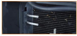
16. Connect the cooler lines to the adapters. Transfer the two safety caps to the new lines.
