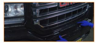
4. Take out the bolts that secure the grille. This includes all hardware along the bottom and top. (8x 10mm bolts)
