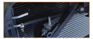
18. Install the short hose to the top port where the holes were drilled and the other to the closer transmissions cooler port. (2x worm gear clamp)
