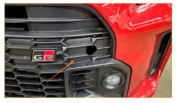
**05.** Insert the tow hook rod through the hole in the tow hook cover and thread it into the tow hook receiver. Tighten with a 19mm socket (or wrench).
