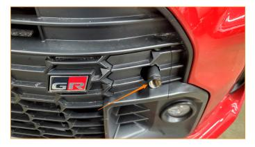
**06.** Thread the tow hook ring onto the rod. With the ring in the desired orientation, use a 25mm wrench to tighten the jam nut. Then, use an 8mm Allan key to tighten the bolt on the side of the ring to fix the position of the ring.
