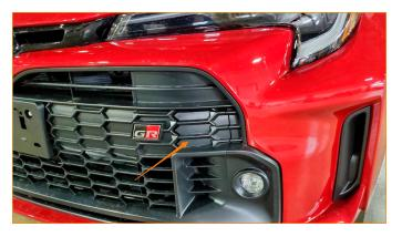
**02.** Disengage the clip attaching the cover to the bumper and remove the cover from the vehicle.
