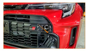
**03.** This step is optional. The tow hook can be installed with the tow hook cover left off the vehicle. Cut out the supplied drilling template and align it on the back of the tow hook cover, as shown below. Using a 1-1/4" hole saw, cut a hole through the tow hook cover in the location marked on the template.
