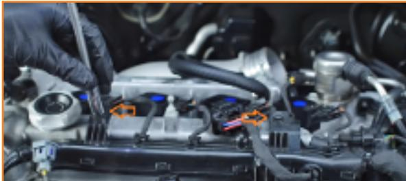
7. Remove the bolt that secures the vacuum line to the intake manifold. (1x 10mm bolt)
