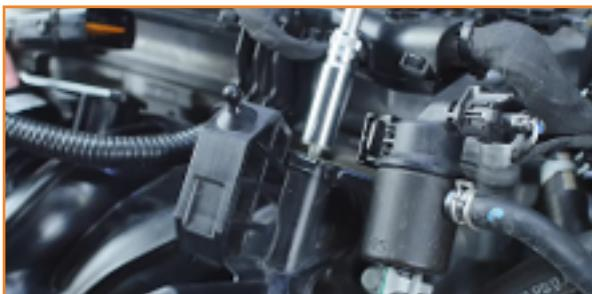
8. Separate the positive terminal on the alternator. (1x 12/13mm nut)
