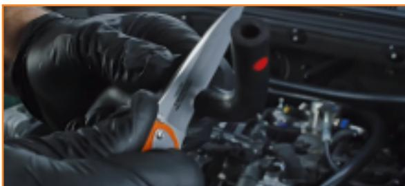
4. Place the smaller side of the fitting into the stock PCV hose. (1x worm gear clamp)
