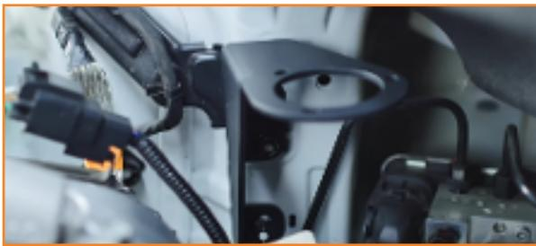
22. Attach the fittings to your catch can. The small fitting goes to the IN port, and the large fitting to the OUT port. Snug them down with a
