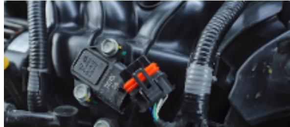
4. Remove the bolt on the bracket that holds the bottom sensors. (1x 10mm bolt)
