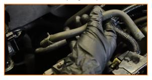
Remove the bolts on the fuel line cover. (2x 10mm bolts)
