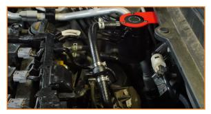
11. Install the inlet hose to the PCV valve and IN port on the catch can. (2x spring clamps)
