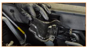
3. Remove the bolts that secure the fuel line bracket. (2x 10mm bolts)
