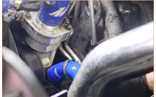
16. Attach the coolant hose to the fitting on the Mishimoto hose, and secure the hose with the original clamp. (1x spring clamp)
