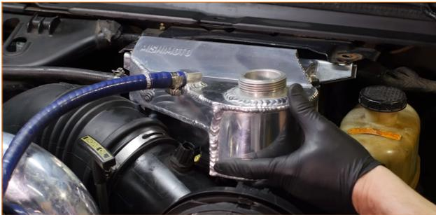
07. Compress the clamp that secures the lower overflow hose to the bottom of the expansion tank and then separate the hose. Then lift the tank out of the way and set it on top of the engine. (1x spring clamp)
