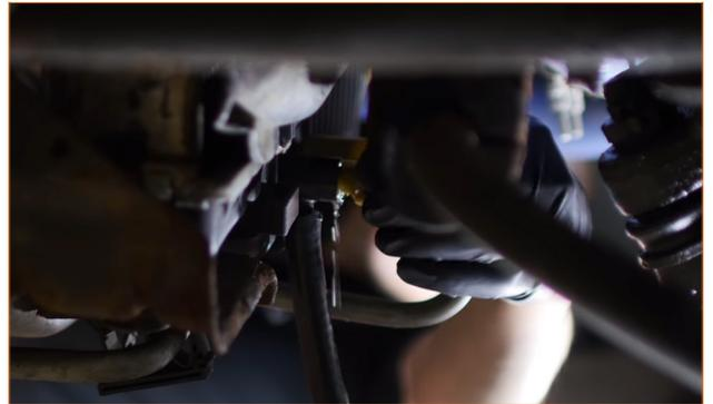
02. The hose we are changing is relatively high in relation to the engine, so you don't need to drain all the coolant. For this install, we drained approximately two gallons from the system. Close the petcock once the desired amount of coolant has been drained.
