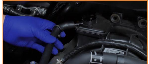
5. Install the smaller hose to the intake port. (1x worm gear clamp)
