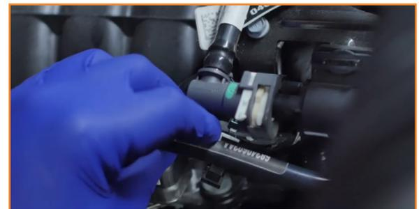
4. Feed the longer hose under the intake and connect it to the PCV valve housing. (1x worm gear clamp)
