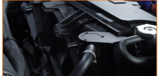
12. Connect the shorter hose to the outlet port on the catch can. (1x worm gear clamp)
