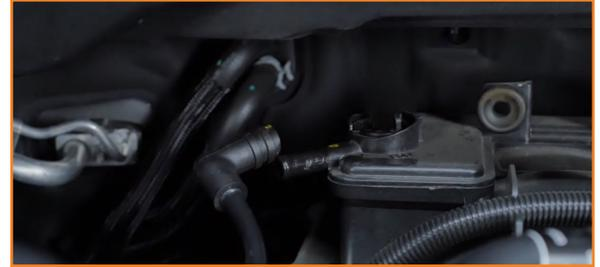
3. Release the tab on the clip that holds the PCV hose. Then remove the hose from the engine bay.
