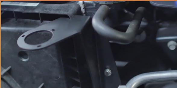
8. Install the additional bracket piece to the back of the catch can bracket. (1x 10mm bolt)
