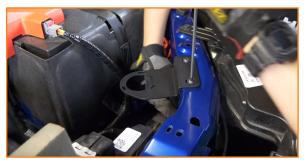
Attach the bend to the inlet port on the catch can. (1x worm gear clamp)
