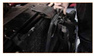
**18.** Reinstall the two 10mm bolts securing the front transmission cooler to the hood release frame.
