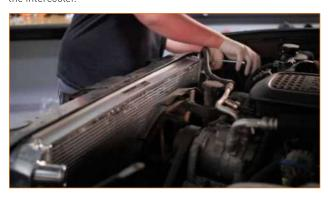
**4.** Now reinstall the transmission cooler lines. These lines feature a quick disconnect, so the clips we removed earlier need to be reinstalled. Once the clips are installed the lines can be pushed back into the radiator. An audible click will indicate that the lines are properly seated in the radiator and clips. Once this is done slide the dust shields back over the fittings.
