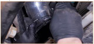
07. Loosen the clamps that secure the Y-shaped induction hose to the airbox and intake pipes. Then separate the induction hose from each connection and remove it from the vehicle. (3x worm-gear clamps)
