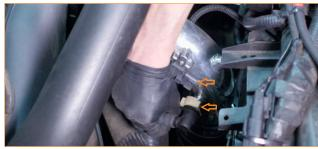
10. Loosen the clamp that secures the cold-side intercooler pipe to the throttle body. Then separate the pipe from the throttle body. Lift the pipe upwards to give yourself more room around the intercooler. (1x worm-gear clamp)
