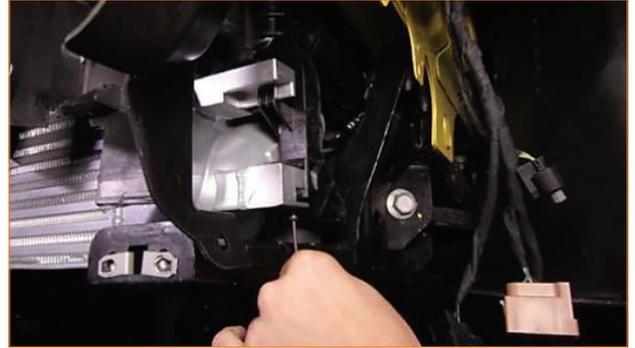
**28.** Tighten the worm-gear clamp on the hot-side pipe. Make sure that the boot is seated all the way on the intercooler. (7mm socket, 7mm socket wrench, or flathead screwdriver)
