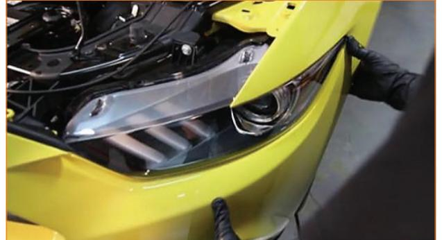
**39.** Reinstall the two 7mm bolts that hold the front fender to the inner fender wall. There is one bolt on either side of the bumper.
