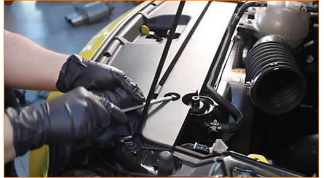
3. Remove the bumper hardware, but do not fully remove the front bumper. (4x pop clips and 6x 8mm screws)
