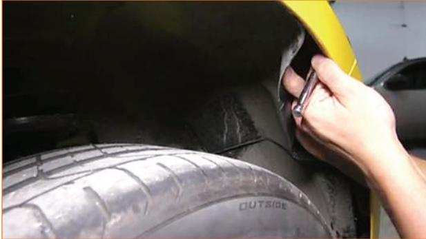
5. Unclip the bumper from the vehicle by pulling the side corners out first, and then lifting the top holes up off the pegs. Once the bumper is loose, unclip the six wire harnesses for the turn signals, headlights, and fog lights. Remove the bumper.
