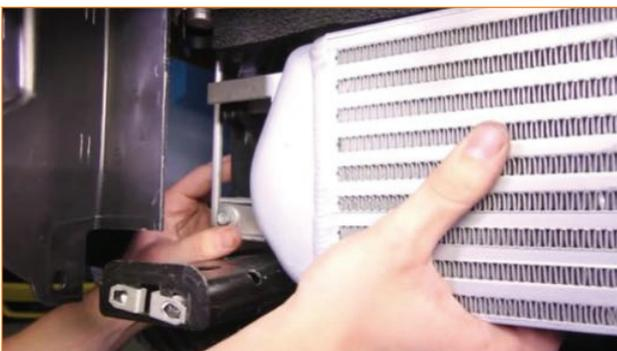
**27.** Install the supplied set screw on the driver side. (1x M4 x 0.7 x 12mm button-head bolt, 1x M4 lock washer, 2.5mm Allen key)
