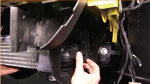
**20.** Lift the intercooler hangers up while pulling forward toward the front of the vehicle.
