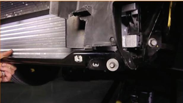
**35.** Reattach the air shutters. Make sure to route the air shutter arm around the front crash beam. The air shutter arm will reattach to the clip on the front air dam. (2x pop clips, 4x 8mm bolts)
