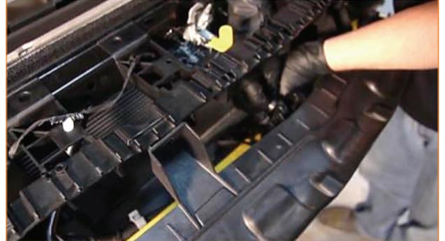
8. Disconnect the wire harness for the air shutter motor.
