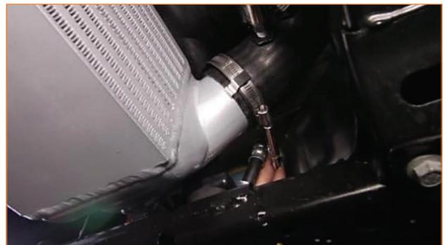
**29.** Tighten the worm-gear clamp on the cold-side pipe. Make sure that the boot is seated all the way on the intercooler. (7mm socket, 7mm socket wrench, or flathead screwdriver)
