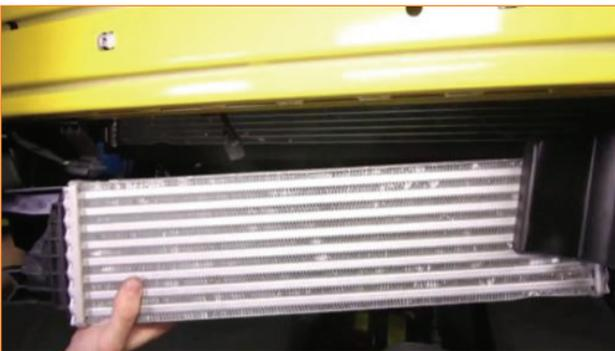
**22.** Remove the MAP sensor from the stock intercooler. (T25 torx bit)
