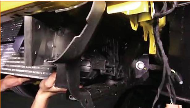
**21.** Once lifted out of the radiator mounts, remove the hot-side coupler while wiggling the intercooler forward. Remove the intercooler.
