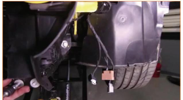
11. Remove the 10mm bolt on the passenger side of the intercooler.
