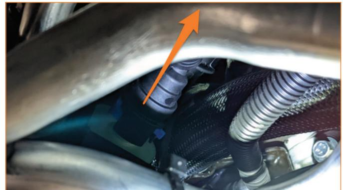
**09.** With both sides disconnected, the PCV line can be removed.
