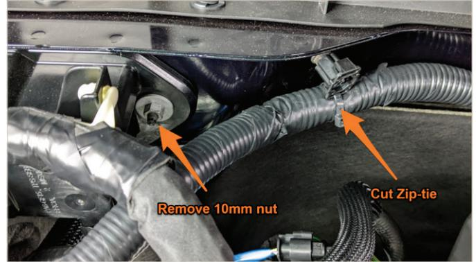
**03.** Unthread the plastic zip tie mount, this part will be reinstalled later.
