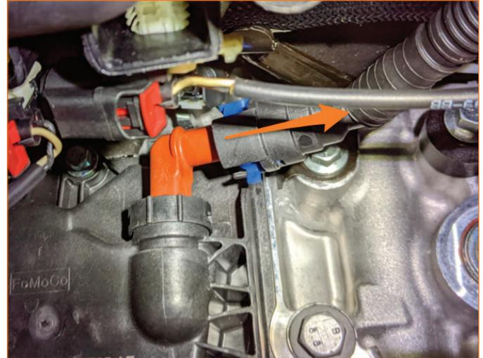
**08.** Remove PCV line quick-disconnect fitting the rear of the intake manifold.
