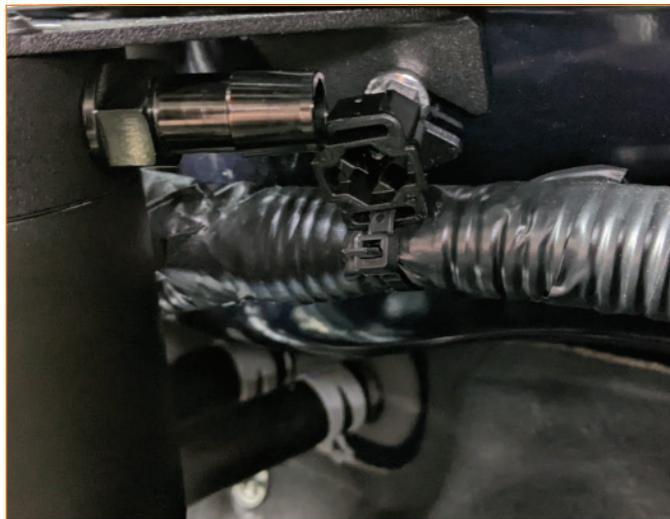
**07.** Remove PCV line quick-disconnect fitting from the air/oil separator located on the left side of the engine block under the intake.
