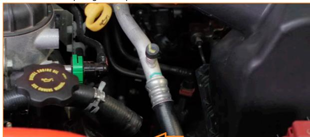
**04.** Compress the clamp that secures the CCV hose to the turbocharger inlet housing and separate the hose from the housing. Then remove the CCV hose from the vehicle. (1x spring-clamp)
