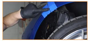
9. Disconnect the headlight washer line on both sides. Have a bucket ready to catch any residual fluid.
