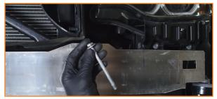
13. Release the tabs and clips to free the shrouding. Remove the shrouding from around the intercooler.
