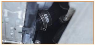
16. Disconnect the cold-side pipe from the intercooler end tank. (1x spring clamp)
