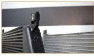
2. Transfer the lower mounting grommets from the factory intercooler to the Mishimoto intercooler.
