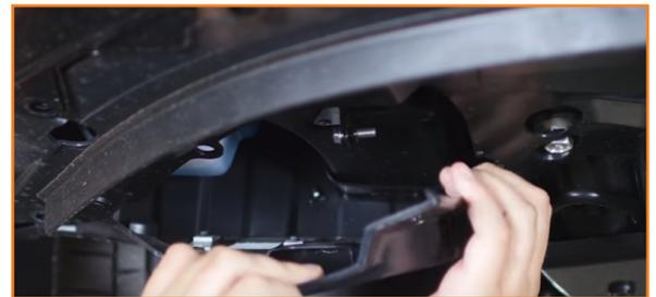
3. Disconnect the fog light on each side once you have access behind the splash shields. Depress the small tab at the end of the connector to separate the connection.
