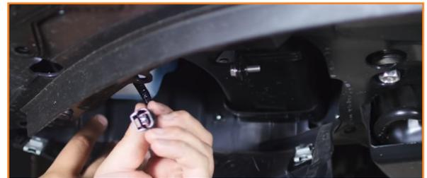
4. Remove the screws that secure the lower edges of the front bumper within the wheel well. (6x Phillips head screws)
