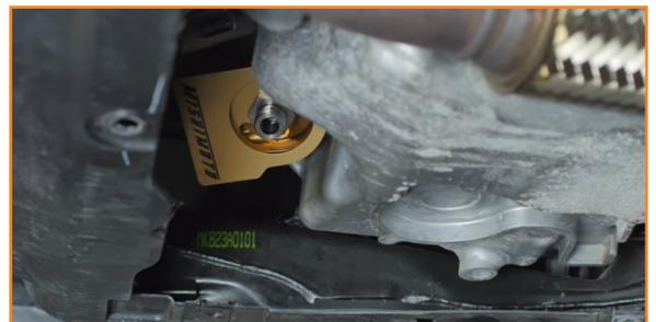
14. Attach the two fittings to your sandwich plate. Snug them down using a wrench. (1" or 10AN wrench)
