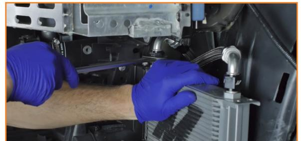
23. Install the shield bracket. Secure the top to the crash beam and the upper edge to the oil cooler. Torque the top bolt to the correct factory specifications. (1x 12mm bolt, 2x 10mm bolts, 2x 10mm nuts)
