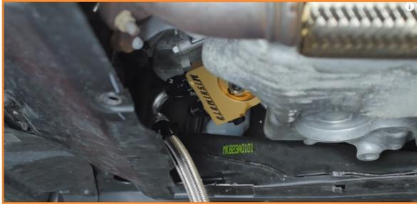
16. Feed the other end of the first line over the frame rail to the front of the driver-side wheel well.
