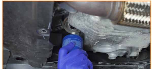
13. Install the sandwich plate using the hardware in your kit. Leave the bolt loose for now. (1x 1-1/16" bolt)
