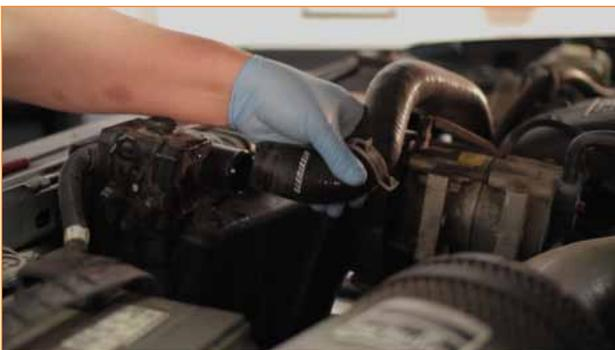
3. Loosen the clamp and remove the upper coolant hose from the radiator.
