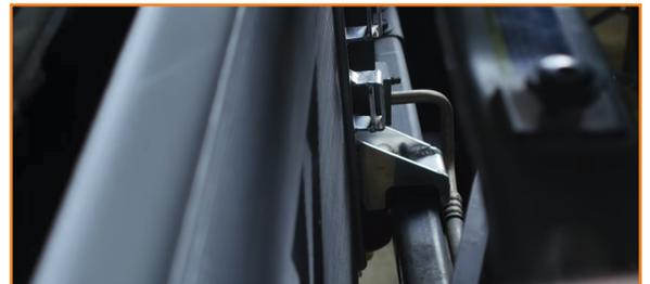
17. Reinstall the transmission cooler using one of the provided bolts from your kit. (1x 10mm bolt)
