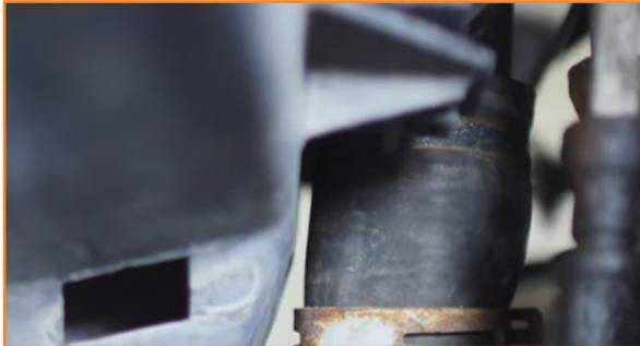
9. Remove the bolts that secure the fan shroud to the radiator and separate the two to give you room to work on taking out the radiator. (2x 10mm bolts)
