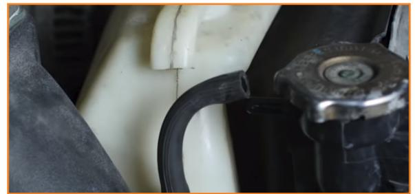
5. Slide the hose off the bottom port on the washer fluid tank. (1x spring clamp)
