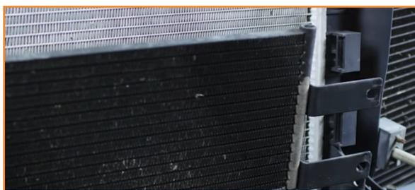
12. Lift the radiator out of the engine bay.
