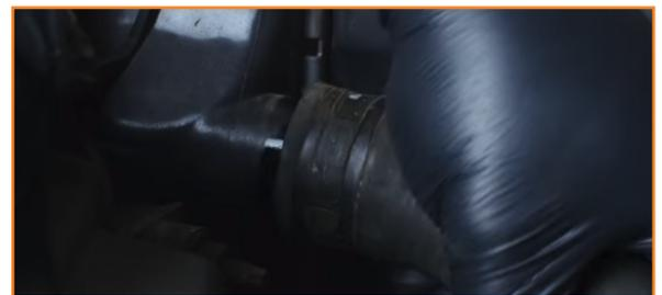
8. Compress the clamp on the lower radiator hose and slide it down the hose. Then pull the lower radiator hose off the port. (1x spring clamp)
