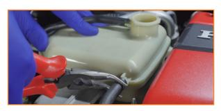
5. Lift the stock tank to reveal the hose connection underneath. Compress the clamp on the hose connection and slide it down the hose. Separate the lower hose underneath the tank. (1x spring clamp)
