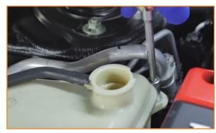
4. Compress the clamp on the upper hose and slide it down the hose. Separate the upper hose from the tank. (1x spring clamp)
