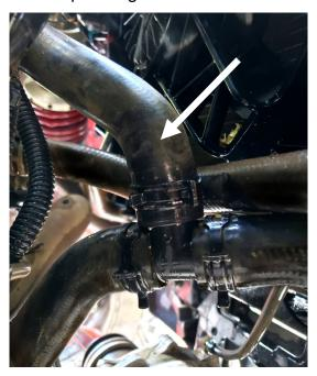
4. Remove the two rubber hoses from the barbed fittings on the front of the coolant tank shown below. Then, using a T30 torx bit, remove the (3) mounting screws securing the tank in position. Additionally the positive lead on the terminal block to the left of the tank will need to be removed.
