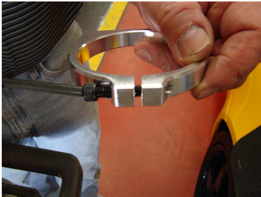
Step 5: Install 1/4-20x1 SHCS as shown in both billet clamps, do not tighten.
