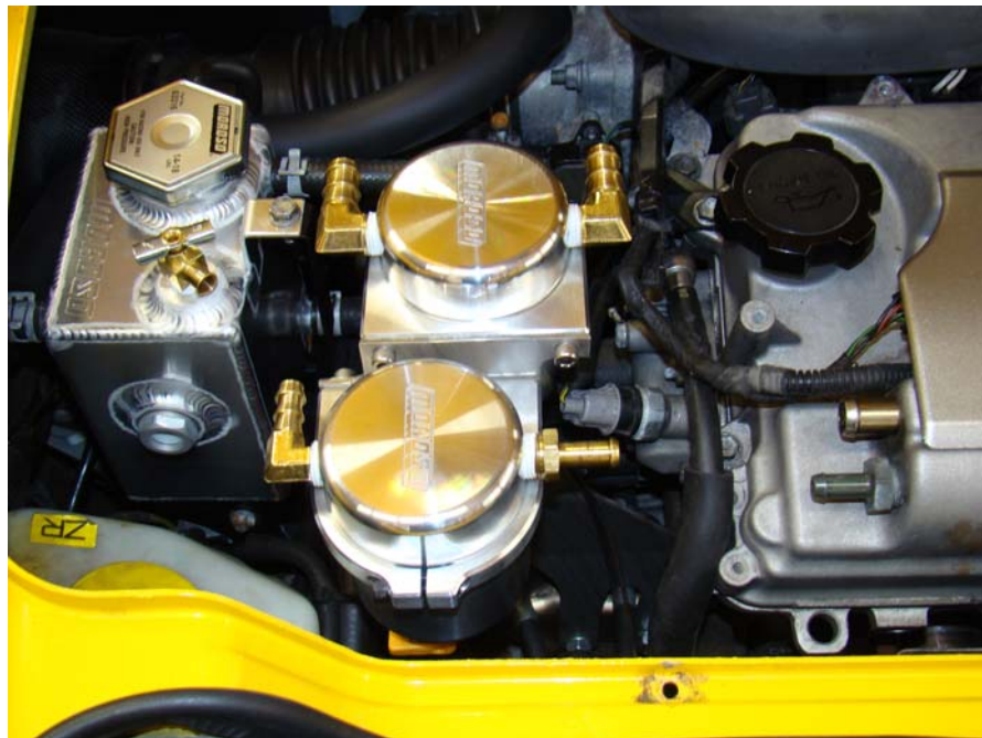
Step 10: Insert Air Oil Separator into rear billet clamp and tighten.
