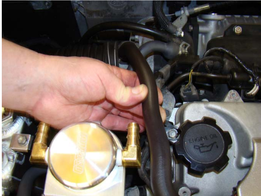
Step 16: Place line next to fitting and mark desired length.
