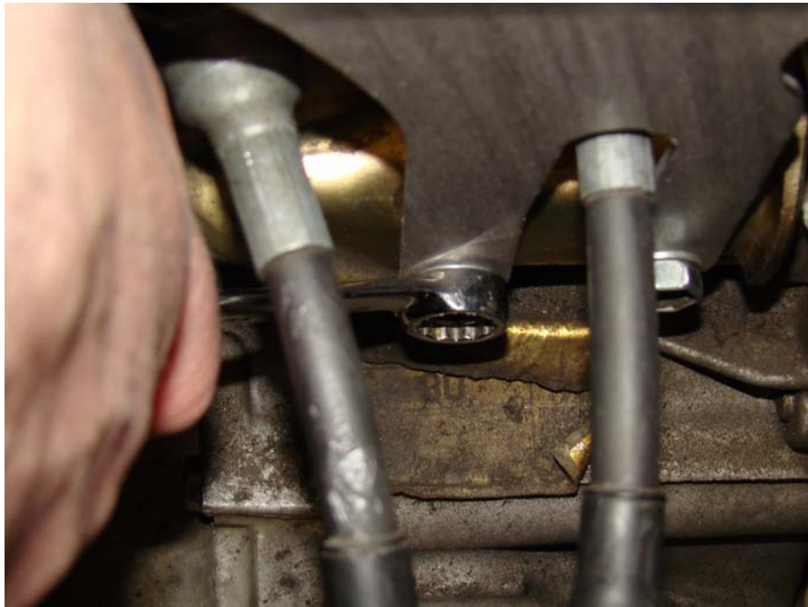
Step 4: Install and tighten stock mounting bolts.
