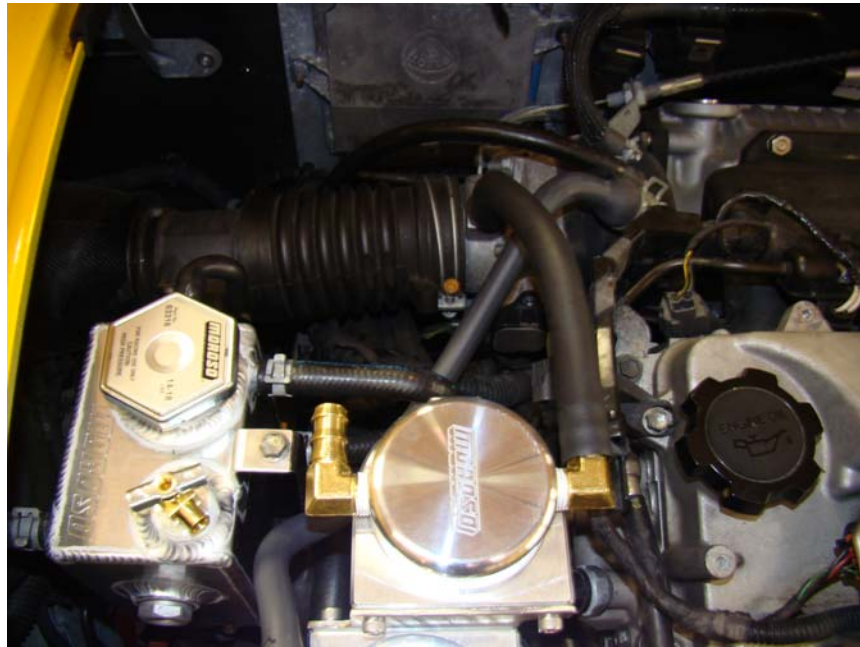
Step 18: Insert line over barbed fitting.
