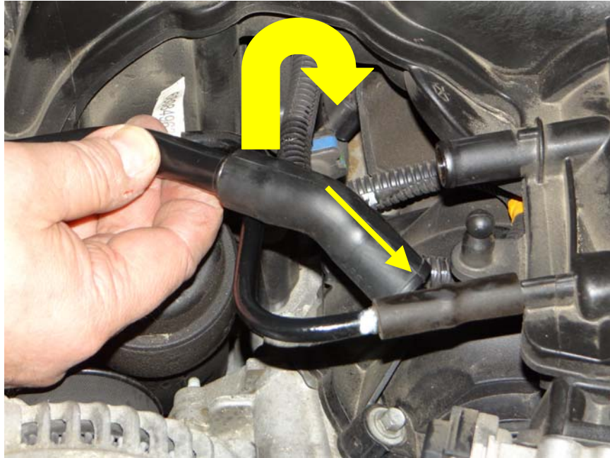
Step 3: Remove from intake nipple and rotate downward as shown.
