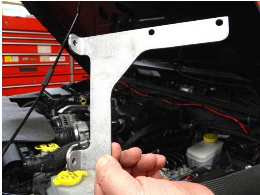
Step 13: Locate stainless mounting bracket from kit.
