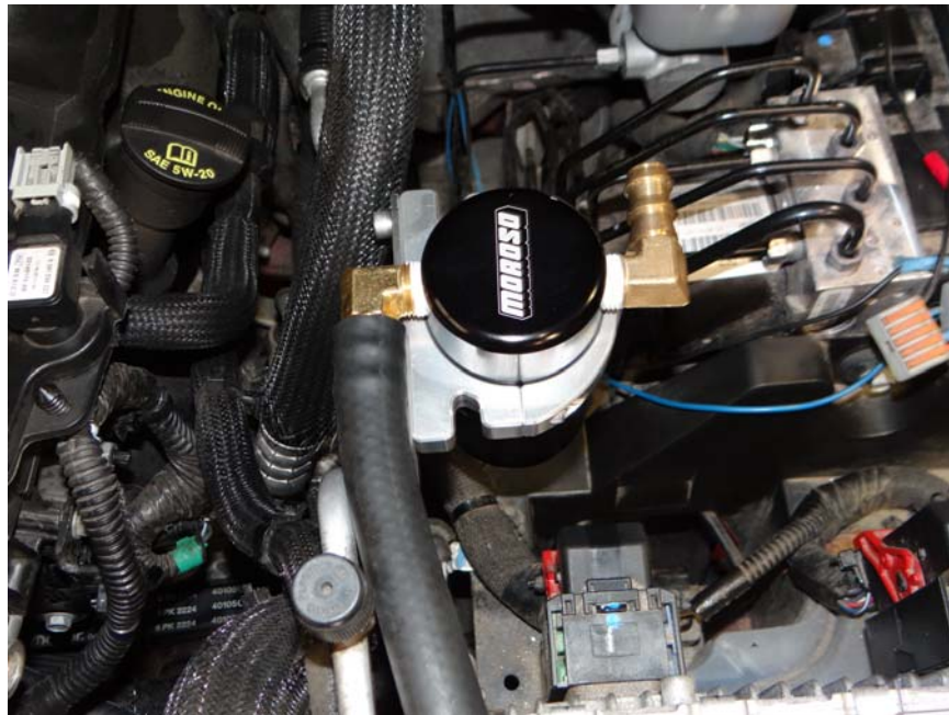
Step 21: Insert hose over nipple.
