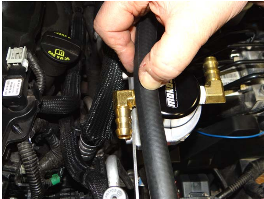
Step 20: Mark hose and cut to length as needed.
