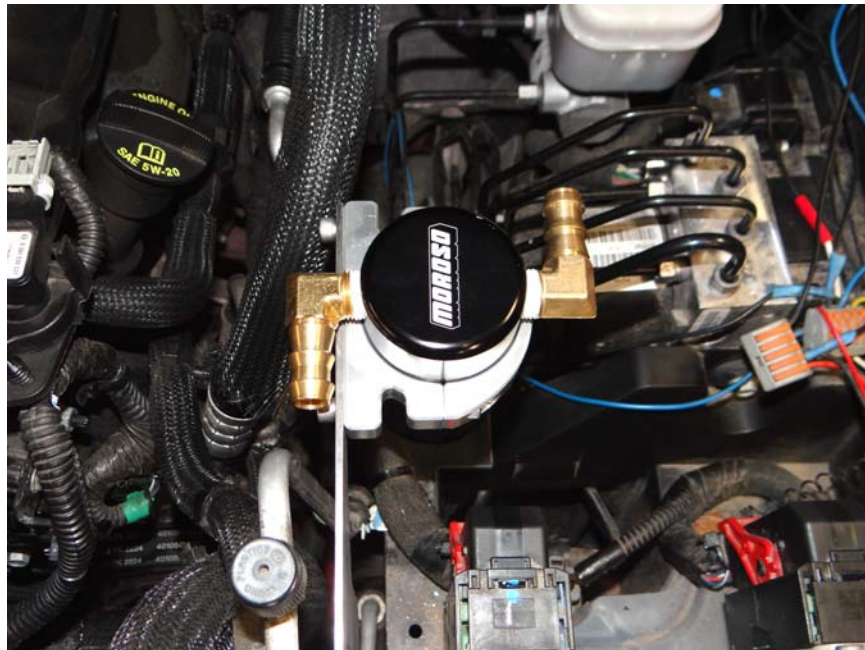
Step 18: Insert Air Oil Separator into billet clamp assembly as shown.
