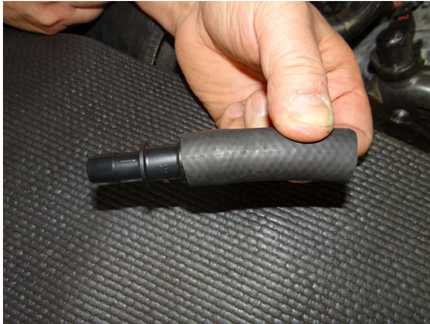
Step 7: Insert coupling into 3" 5/8 hose provided in kit.
