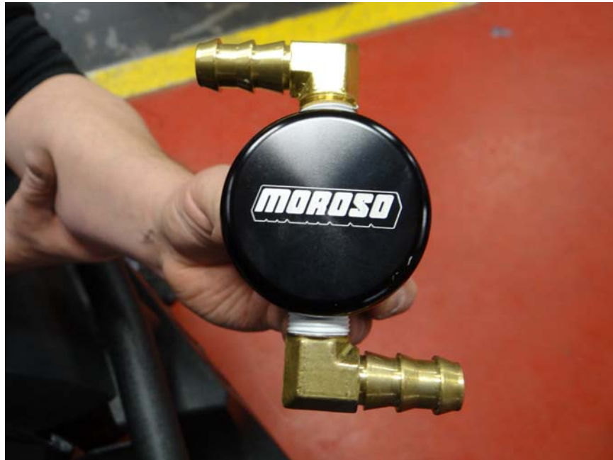
Step 17: Assemble air oil separator as shown using Teflon tape on fittings.
