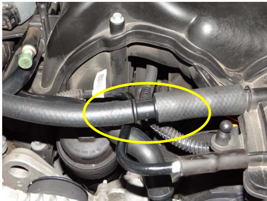
Step 9: Using 60" length of hose provided in kit insert over coupling.
