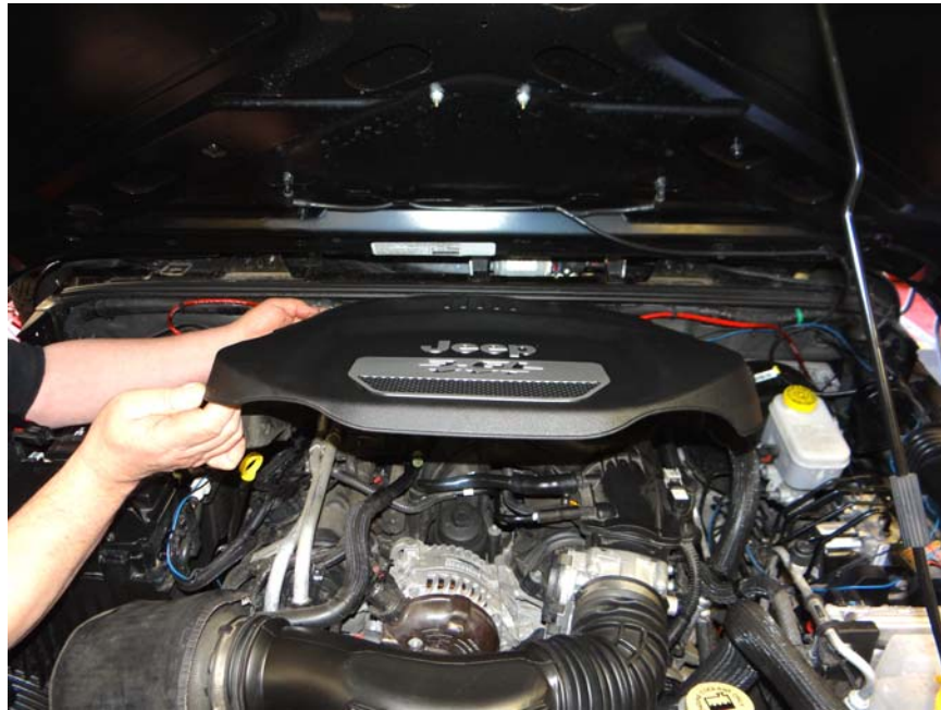
Step 1: Remove intake cover.
