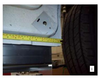
Measuring from the front wheel well back, Fig 1 mark the following locations on the pinch weld. There will be factory holes in line with these marks that will be used to mount the running board brackets
