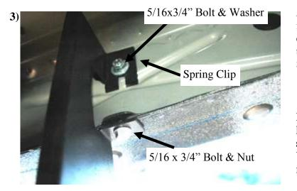
Attach brackets to vehicle by inserting a 5/16" x 3/4" bolt into the spring clip and 5/16" x 3/4" bolt and nut through the pinch weld hole. And 8mm bolt on GMC models.
