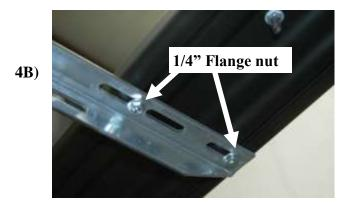
Place the board on the brackets and center up on the cab of the vehicle from front to rear. Attach to the brackets using #14 X 3/4" long self drilling screws.
