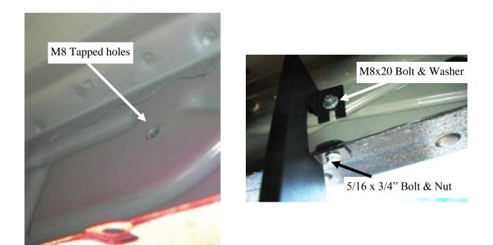
On some models you will find tapped hole in the locations for the bracket. With these use the M8 bolt through a flat washer to secure the top of bracket to the rear of the rocker panel as shown in photo.
