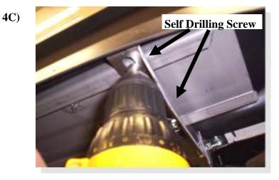
Place the board on the brackets and center up on the cab of the vehicle from front to rear. Attach to the brackets using #14 X 3/4" long self drilling screws into the shoulder of the steel channel on the bottom of the board.
