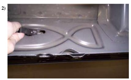
Remove the round plastic cap covering the large hole with a screw driver located on rear of the rocker panel. Slide a spring clip into hole until it snaps into the other hole.
