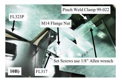
Slide the FL317 bracket up onto the M14 threads on the front bed cross brace. Thread the M14 flange nut onto the threads tighten completely, making sure the FL317 is slid all the way back in top slot use 21mm deep socket or 13/16" if a metric socket is not available.
