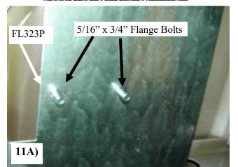
Place two 5/16" x 3/4" flange bolts down through the holes in the FL323P from the top, so the threads point downward shown in photo 11A
