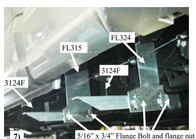
Mount the 3124F angles to the FL315 and to the FL324 lower slots with 5/16" x 3/4" flange bolts and flange nuts through each slot as shown in photo 7
