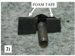
Place a strips of foam tape on both sides of the threads of the 30-3410 stud plates as shown in photo above, this will insulate the steel bracket from the aluminum body to avoid corrosion.
