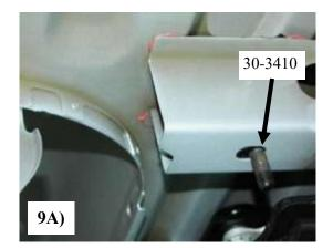
Slide the 30-3410 stud plate into the second bed cross brace so that the threads drop down through the slot in the cross brace as shown in photo **9A**
