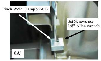
Place a 99-022 pinch weld clamp up onto the pinch weld as shown in photo **8A**, this will be at 4 1/8" from the front of were the pinch weld starts to the center of the 99-022. photo **8B** Tighten the set screws as tight as possible by hand to secure clamp onto the pinch weld. Make sure the set screws are located on the inside of the vehicle tightening outward as shown in photo **8A**
