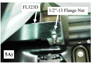
Slide the FL323D up over the threads of the 30-3410 stud plate and place a 1/2-13 flange nut onto the threads to secure. Photo 5A
