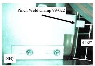
Use pair of vice grip pliers to hold the 99-022 when tightening the set screws, this will give better leverage.
