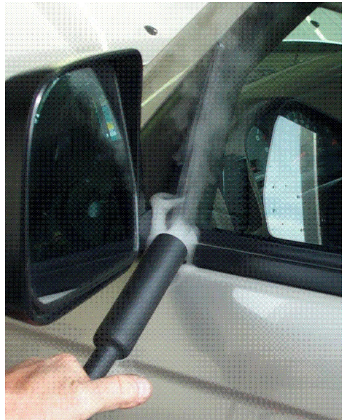
Vapor disturbance pinpoints leak.
