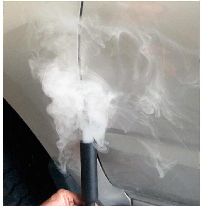
No vapor disturbance indicates no leak.
