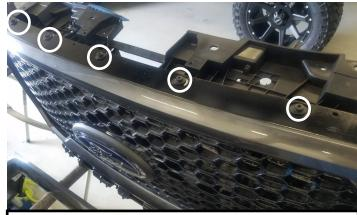
7. Remove (5) fasteners using a clip removal too.
