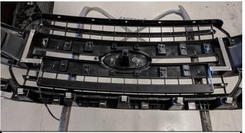
13. Set the grille face down on something soft and lay the combined bracket and light bar assembly onto the studs in the grille.
