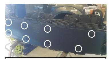
10. Remove (8) clips holding rubber cover on bottom of the assembly.
