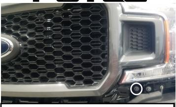
6. Remove (2) 8mm bolts. Pull grille to unclip fasteners and remove assembly. Driver side shown.
