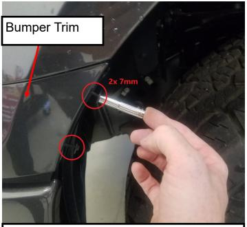
4. Remove (2) 7mm bolts in each front fender well. **If the vehicle is equipped with fender flares,** remove clips inside wheel. Pull fender flare out to disengage from bumper trim piece.
