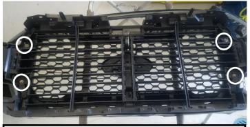
8. Remove (4) 10mm nuts holding active shutter assembly to grille.
