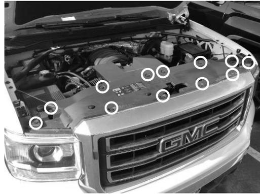
7. Remove plastic cover by removing 12 retaining clips with flat head screw driver (locations shown above).
