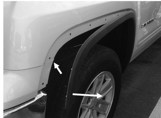
3. Pull front of fender trim away from truck. Remove (1) 7mm bolt from inside of upper bumper, location indicated by arrow. Driver side is shown. Repeat on passenger side.
