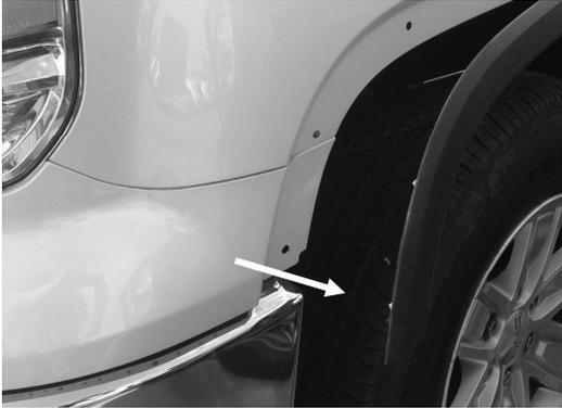
4. Pull out upper bumper end. Driver side is shown. Repeat on passenger side.
