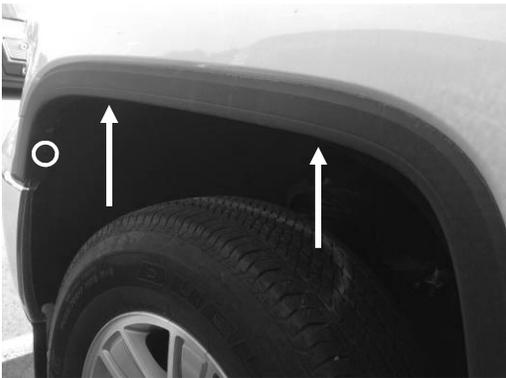
2. Remove (2) T15 Head Bolts (shown by arrows) and (1) 7mm bolt (shown by circle) from the front fender trim of truck. Driver side is shown. Repeat on passenger side.
