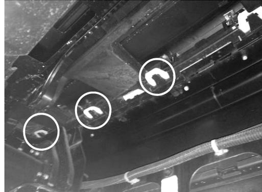
5. On back side of bumper, use a flat headed screw driver to unclip (total 6) clips. Driver side locations shown above. Repeat on passenger side
