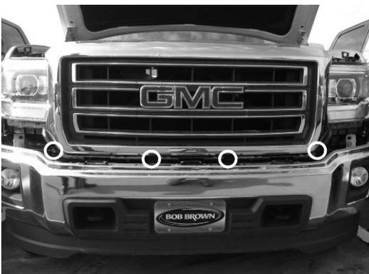
8. Remove (8) 10mm bolts from the grille. Locations shown above. Once bolts are removed pull grille straight off of truck.
