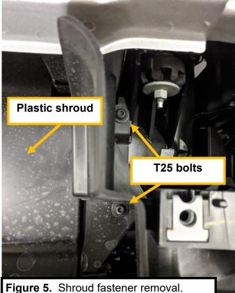
**Figure 5.** Shroud fastener removal. Driver's side viewed from above.
