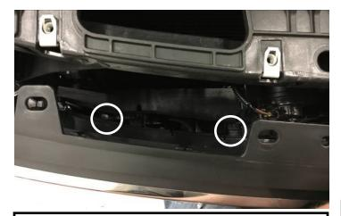
3. Pull upper grille forward to release upper grille clips. Once out, release 4 bottom clips with a flat head screwdriver. Passenger side locations are shown. Repeat on driver's side.
