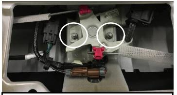
2. Remove (2) 10mm bolts and shift latch assembly out of the way. This allows for better access to the back side of the emblem.
