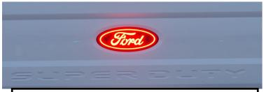
9a. Test the emblem. It is tied to the running lamps and should be on when the Daytime Running Lamps or head lights are on. Zip-tie wires into place, making sure the wire is protected from pinch points and sharp edges.
