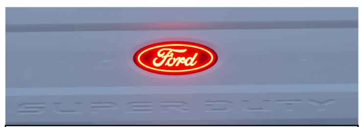
7. Test the emblem (key on or vehicle running) before reassembling. Zip-tie wires to existing wiring harness. Keep the wire clear of sharp edges and from interfering with latch mechanism.
