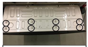
1. Lower tailgate and remove the eight T-30 screws from the access cover. Remove access cover.
