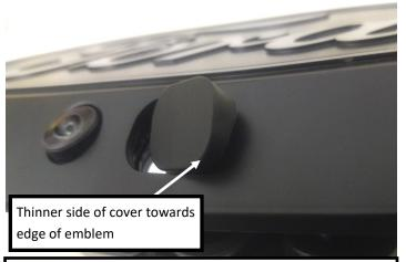
8. Front camera equipped trucks: Apply 3M tape to back of included washer cover. Peel backing off and press onto factory washer cover. Make sure orientation is correct!
