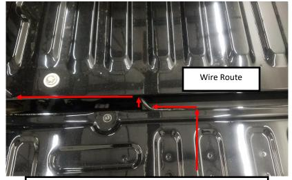
7a. Feed LED emblem wires to driver's tail lamp harness. Follow existing harness coming out of tailgate. Route the wire under the vehicle, behind the bumper, and up into the tail lamp cavity. Protect the wire with split loom or abrasion resistant sleeving.
