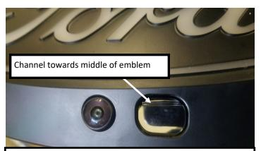
7. **Front camera equipped trucks:** Reinstall nozzle cover, ensuring proper orientation. Needle nose pliers may be needed to pull nozzle arm through opening when installing nozzle cover.
