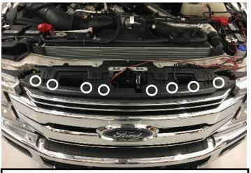
2. Once cover is removed, remove the top 8 grille screws with 10mm wrench (location shown above).
