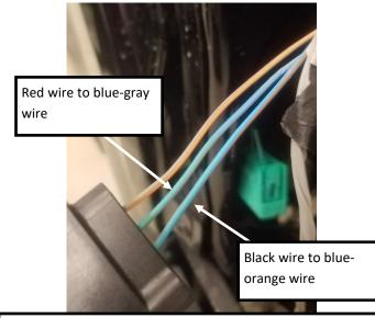
8a. Using provided ScotchLoks, splice the wires into tail lamp harness. Hook the emblem red wire to the blue gray wire, and the emblem black wire to blue orange wire.
