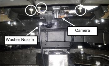
4. Disconnect camera harness and washer nozzle, if equipped. Remove grille and place on flat surface. Be careful not to damage the front of the grille. Remove (3) 10mm nuts to release emblem.
