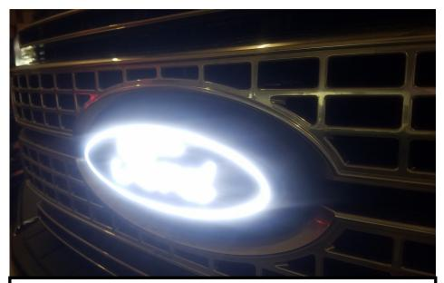
14. Test the emblem (key on or vehicle running). Make sure to zip-tie wires safely in place before final reassembly.
