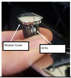
5. **Front camera equipped trucks:** Remove (2) T25 torx screws mounting camera assembly to emblem. Remove spray nozzle cover by gently prying arms with flat head screwdriver.
