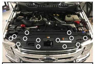
1. Remove plastic cover by removing 13 retaining clips (number of retaining clips may vary) with flat head screw driver (locations shown above).
