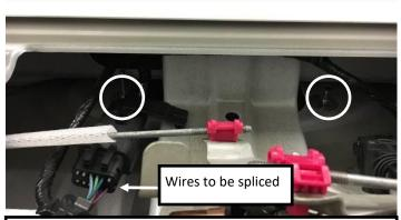
5. Install the emblem into the tailgate using the provided flange nuts. **Be careful not to overtighten the fasteners and damage the tailgate.**
