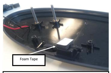
6. **Front camera equipped trucks:** Apply 3M foam tape to back of camera to prevent vibration in housing. Reinstall camera and washer nozzle mounting assembly using original T25 torx screws.
