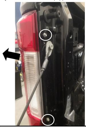
6a. Remove (2) 8mm bolts from driver's tail lamp. Pull out on tail lamp (away from fender) to remove from vehicle.
