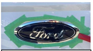
3. The emblem is held by 2 plastic clips and adhesive tape. Carefully pry on emblem and push the clips from inside the tailgate. **BE CAREFUL NOT TO DAMAGE THE PAINT OR SHEET METAL.**
