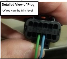
6. Using provided ScotchLoks, splice the emblem red wire into blue wire of the harness (pin 10). Splice the emblem black wire into the green wire of the harness (pin 9). This is easier with the plug disconnected.
