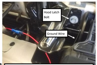
13. Connect Add-A-Fuse harness to red wire from LED emblem. Strip ~1/2" of insulation from black wire, and ground to chassis. For example, loosen (do not remove) the 10mm bolt holding hood latch enough to wrap black ground wire around bolt. Tighten bolt, making sure wire is secured.
