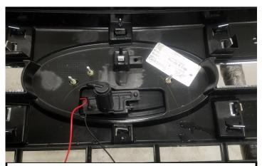
9. Install emblem onto grille with provided (3) flange nuts. Tighten with 8mm wrench, being careful not to overtighten.
