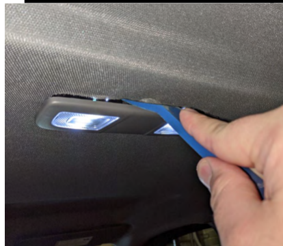
Figure 3: Cargo light removal
