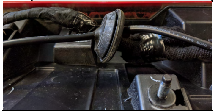
Figure 10: Wire routing through grommet
