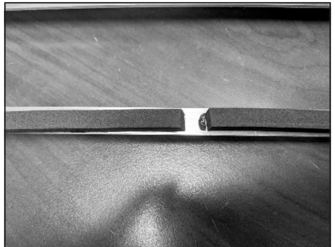
Figure 4: Cutting slot in gasket.
