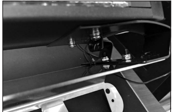
Figure 1: Installing Hornet Light onto bracket.
