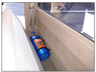
Figure 4 Bottle with blow down tube installed
