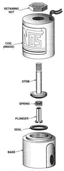
Figure 18 Exploded View of a Typical Solenoid
