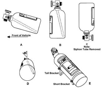
**Figure 3 Nitrous Bottle Mounting Orientations**
