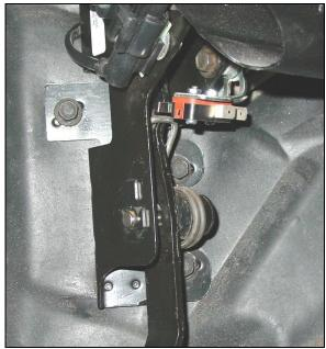
Figure 16 Microswitch in completed location
