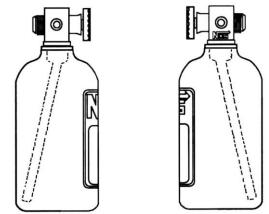
Figure 2 Nitrous Bottle Siphon Tube Orientation
