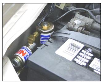
Figure 11 Completed solenoid mounting
