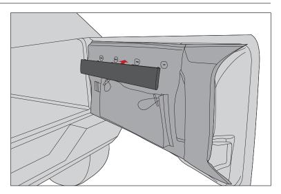
5. Remove adhesive backing from tape. Pull edges of Tailgate Cover tightly over tailgate and press firmly to adhere to tailgate.
