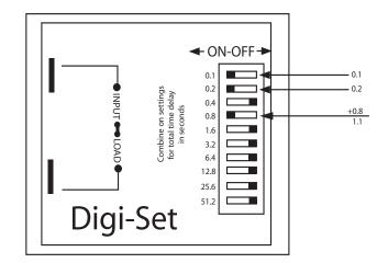
This time delay switch is set to activate a second stage of nitrous after a delay of 1.10 seconds
