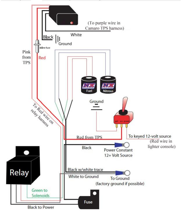
Attach the white wire of the TPS module wire to the purple wire of the Camaro throttle body harness (AKA TPS Wire). NOTE: The TPS module will be mounted inside, so you should route the white wire from the TPS module through the previously mentioned firewall grommet. Make sure to solder and tape the connection.
