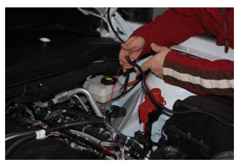
Attach the white wire of the NX relay harness to ground (optionally through a fuel pressure safety switch). Connect the black wire of the NX relay harness to the positive battery stud on the driver's side of the engine bay
