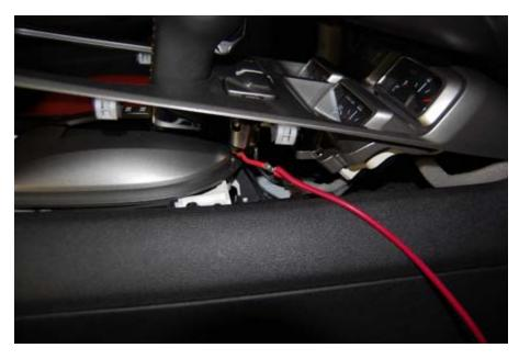
13. Choose a suitable location for the master arming switch to be mounted; the switch will need to be accessible from the driver's seat. (we chose to place our master arming switch in the A-pillar).
