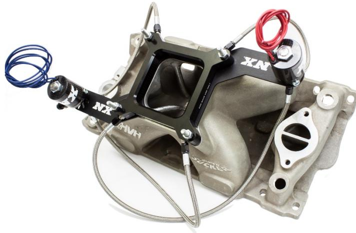
NOTE: As you can see in the (Illustration B), the fuel and nitrous ports on the plate are on opposite corners of each other. Please advise when installing the lines on the plate and make sure they are installed on the right ports for you solenoids.
