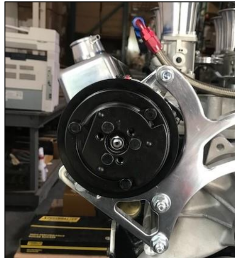
Figure 10: Air compressor installed in the correct location.
