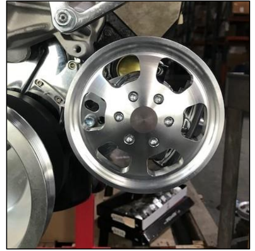
Figure 16: Power steering pulley installed with the 6mm socket head cap screws firmly tighten.
