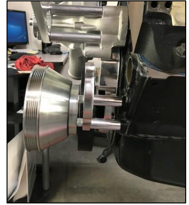
Figure 12: Power steering bracket mounted correctly
