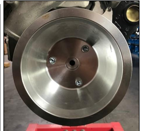
Figure 8: Side view of the crank pulley/spacer assembly
