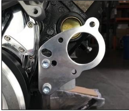
Figure 12: Power steering bracket mounted correctly
