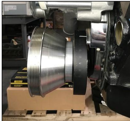
Figure 8: Side view of the crank pulley/spacer assembly
