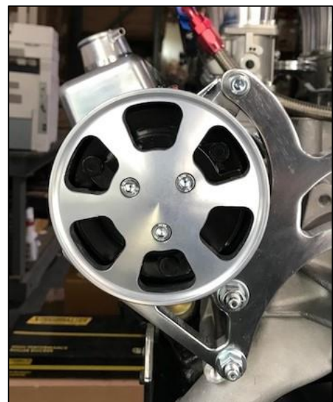
Figure 11: Air compressor cap installed
