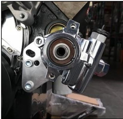
Figure 14: Front view of the power steering pump mounted on the bracket.
