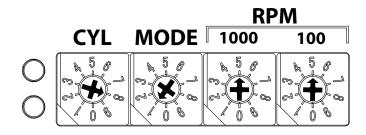
**Note:** Setting a rev limit values less then 1000 RPM requires that the "**1000**" switch be placed in the 0 position. For a maximum rev limit of 10,000 RPM both "**1000**" and "**100**" switches would be in the 0 position.
