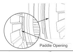
**18.** Insert an active spacer into a driver. Seat the spacer paddle at the missing extended tooth.
