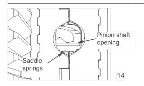
**34.** Keeping both drivers fully engaged, rotate both wheels back 1/4 turn to expose pinion shaft opening. Make sure saddle springs are all fully seated.
