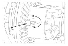
**37.** Insert retaining bolt/roll-pin into case/shaft.
