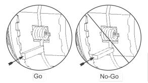
**32.** Check the gap between drivers using check block. The narrow side of the block should fit inbetween drivers, but the wider side should not fit.
