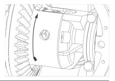
**36.** Using the retaining bolt/roll-pin as a handle, insert the shaft into the differential. Press hard while twisting to pass shaft by springs.
