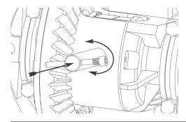
**38.** Using the retaining bolt/roll-pin as a handle, insert the shaft into the differential. Press hard while twisting to pass shaft by springs.
