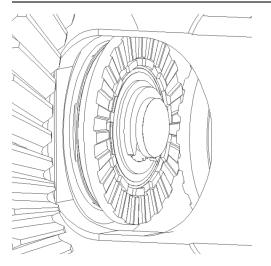
**15.** Install c-clip on ring gear side axle shaft only.
