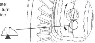
**29.** Compress inner spring and install the second spring assembly into the second spring slot.
