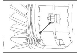
**26.** Compress inner spring and install spring assembly into spring slot.
