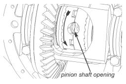
**36.** Feel through pinion shaft opening and verify both spacers and drivers are fully seated onto couplers. Verify all 8 saddle springs are fully seated in holes.
