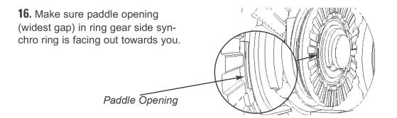
**17.** Insert the non-slotted spacer into the non-slotted driver. Seat the spacer paddle at the paddle opening in driver (missing extended tooth).
