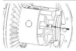
**39.** Insert retaining bolt/roll-pin into case/shaft. Tighten retaining bolt firmly.
