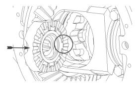
**23.** Verify spacer paddle is aligned with the paddle opening in synchro ring and press down on driver/spacer to seat on coupler; driver teeth should be fully engaged all the way around.
