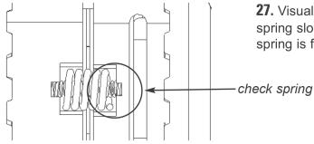
**27.** Visually inspect notches in spring slot to make sure inner spring is fully seated.
