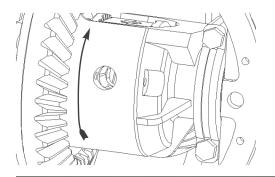
**37.** Keeping couplers and drivers stationary, rotate case 1/4 turn forward to align pinion shaft opening with driver saddles.
