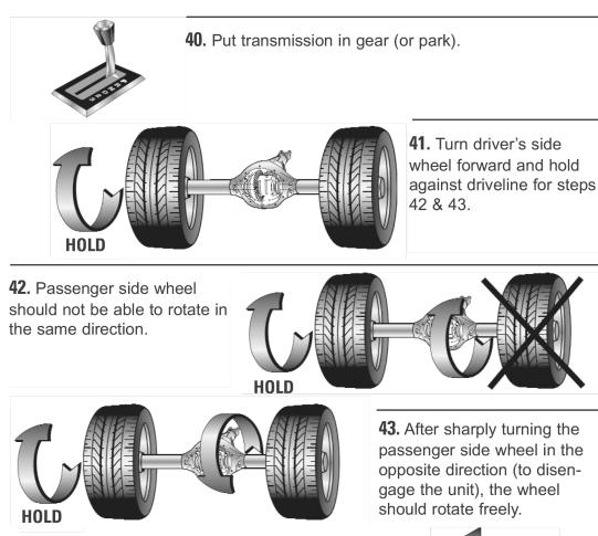
. Repeat the test for both wheels in both directions.
