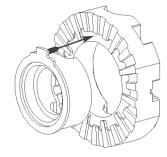
**18.** Insert driver/spacer as shown, making sure spacer paddle is facing out towards you.
