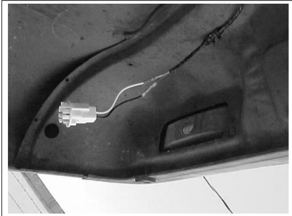
Figure 7.12 Turn Signal has been spliced to the harness and ready to install.
