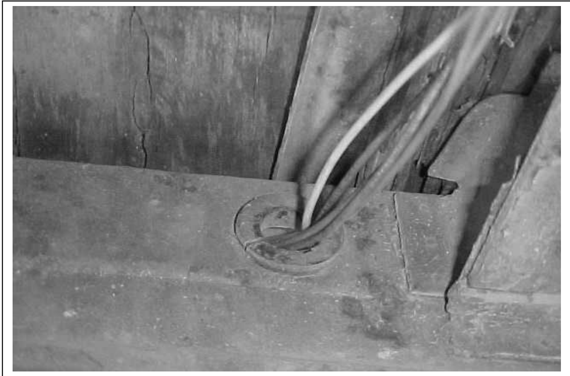
Figure 6.5 The cross-member at the rear of the truck has a hole and grommet to route your tail light wires through.
