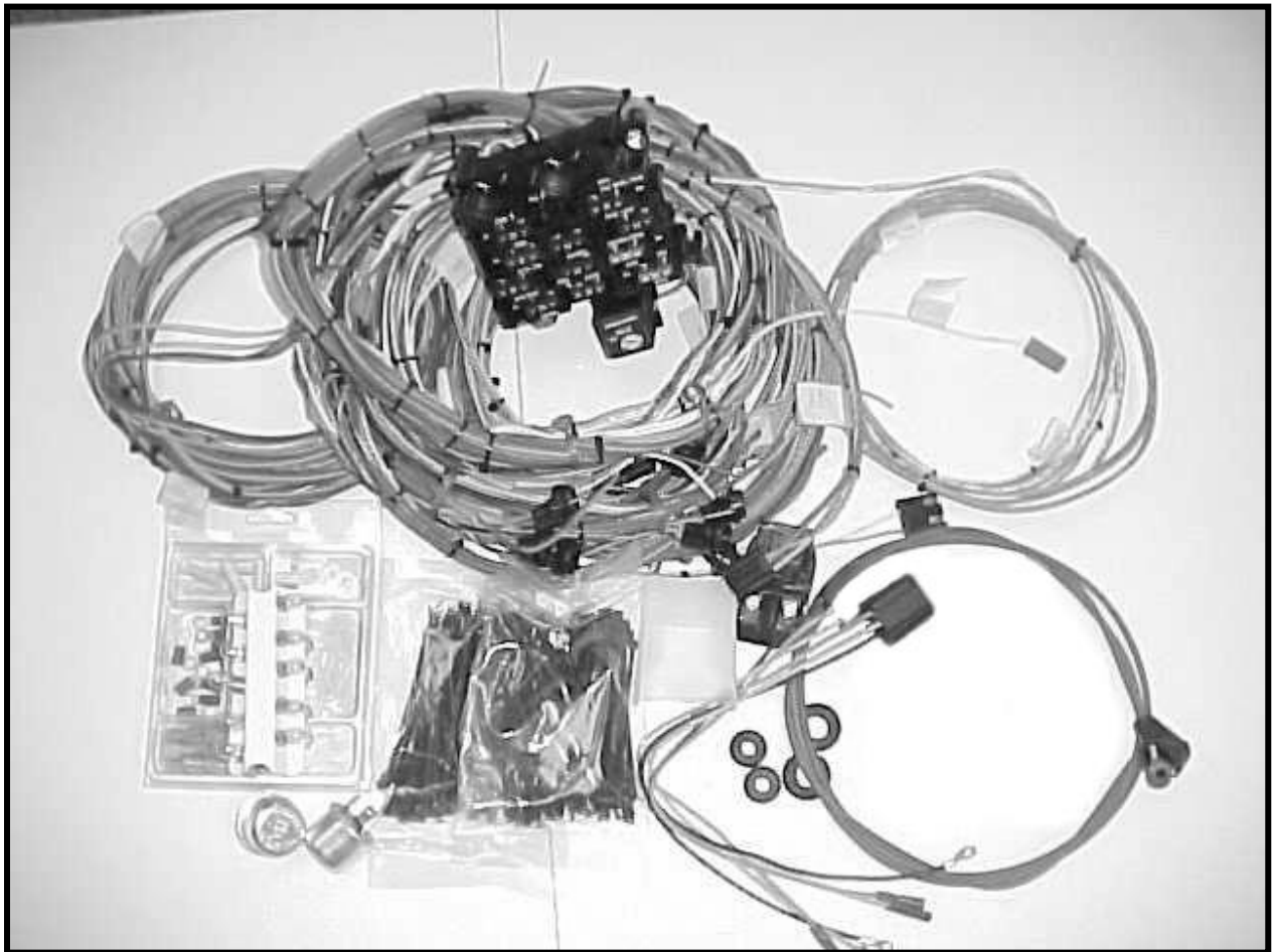
Figure 3-1 The Painless Performance Wire Harness Kit (Part #10112)
