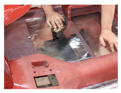
Repeat step until firewall is completely covered. HushMat Ultra is proven to remove a minimum of 40% of the thermal transfer penetrating the firewall. If the pre-HushMat treatment thermal transfer is greater than 180 degrees F, you will need to install Silencer Megabond ½" directly on top of the HushMat Ultra. Follow the same process of planning the Silencer Megabond on the surface and trace any necessary cut-outs prior to removing the release liner.
