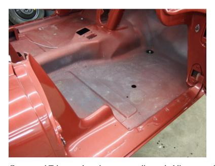
Remove Seats, Carpet, and Trim panel sections surrounding or holding carpet in place. Remove carpet pad and any loose foam pieces down to the floor pan. There is no need to remove the factory damping material.
