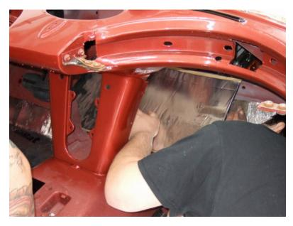
Start at one straight edge (side or top of firewall as far under instrument panel as possible. If restoring a street rod and hot rod and no trim or instrument panel is in vehicle then start at the top of the firewall just under the windshield frame. IF the instrument panel is installed reach as far up firewall as possible.
