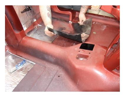
Using a razor knife or scissors cut out all necessary areas. Then peel back the release paper at one side and place it directly on the sheet metal. Apply uniform hand pressure to the sheet and peel back the release paper from underside plying pressure as you progress across the sheet. IF any air-bubbles form under the sheet poke the center of the air bubble with you knife and press sheet down to surface allowing entrapped air to escape.
