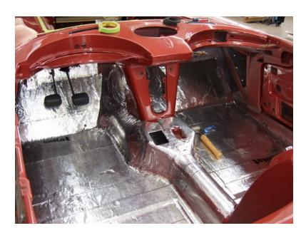
Proceed with the same application process across the entire floor pan and over the transmission tunnel. On the flat or horizontal sections of the floor pan you can install Silencer Megabond ¼". On the tunnel and firewall we recommend ½". The combination of HushMat Ultra and Silencer Megabond should reduce thermal transfer by over 55%. This is done with less than 0.57 pounds per square foot applied.
