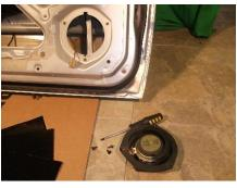
Step 2: Peel brown release paper on one sheet of HushMat Ultra (Part #10110) and apply over speaker opening as shown. Trim out center of sheet exposing the mounting hole.
