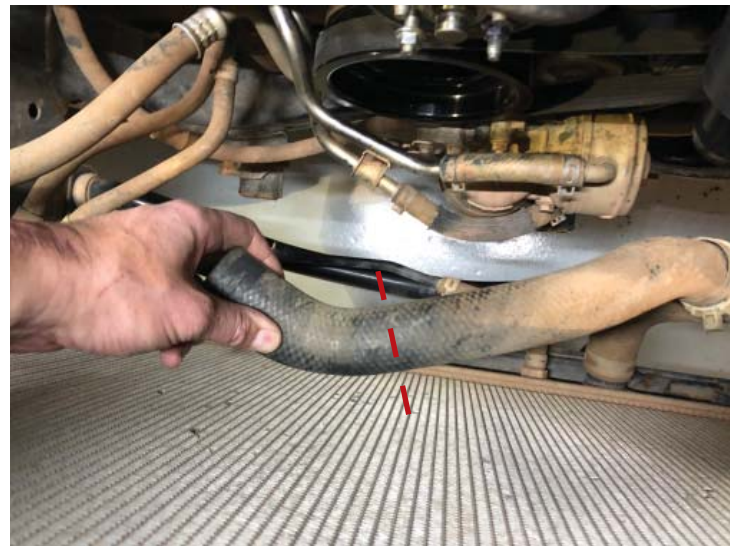
Cut Hose At Line
