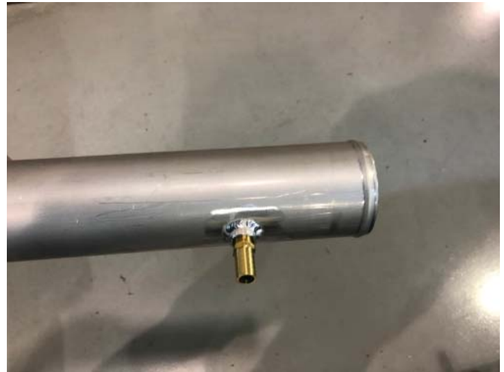
Barb Fitting Installed Into Inlet Tube
