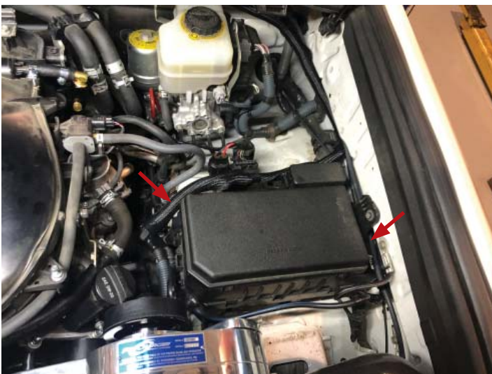
Route Cables Behind Fuse Box
