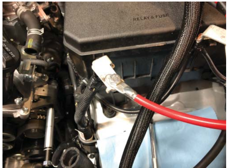
Battery Cable Installed
