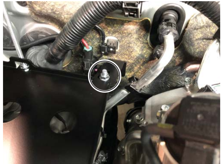
Carriage Bolt Installed
