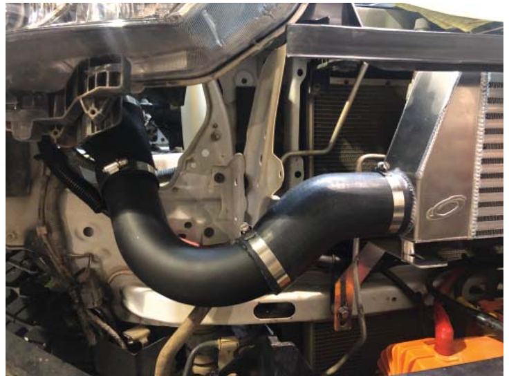
Tubing Out Of Intercooler Installed
