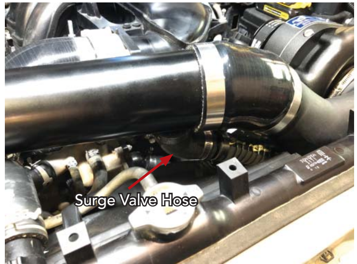
Surge Valve Hose Connected To Inlet Tube
