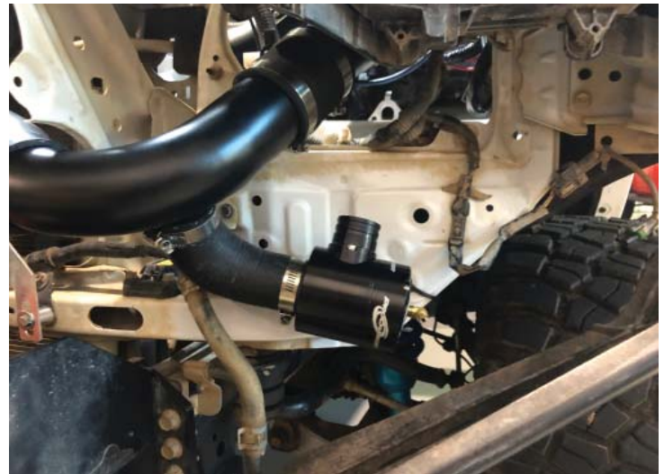
Surge Valve Installed
