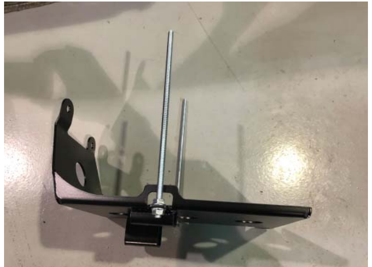
Studs Mounted To Battery Tray
