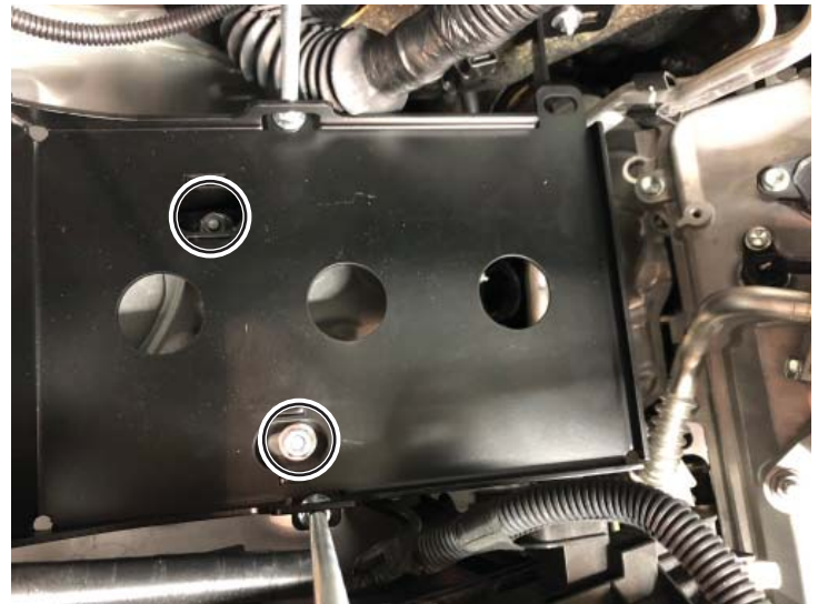
Nuts Installed Over Studs
