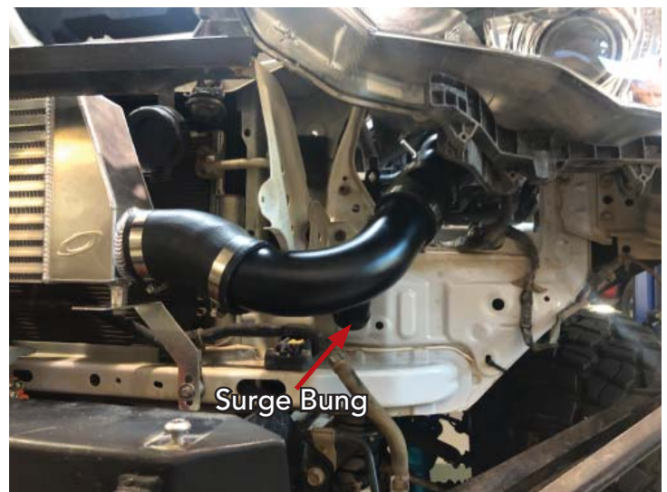
Tubing To Intercooler Installed
