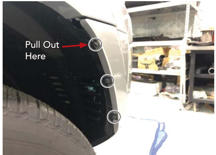
Wheel Well bolts
