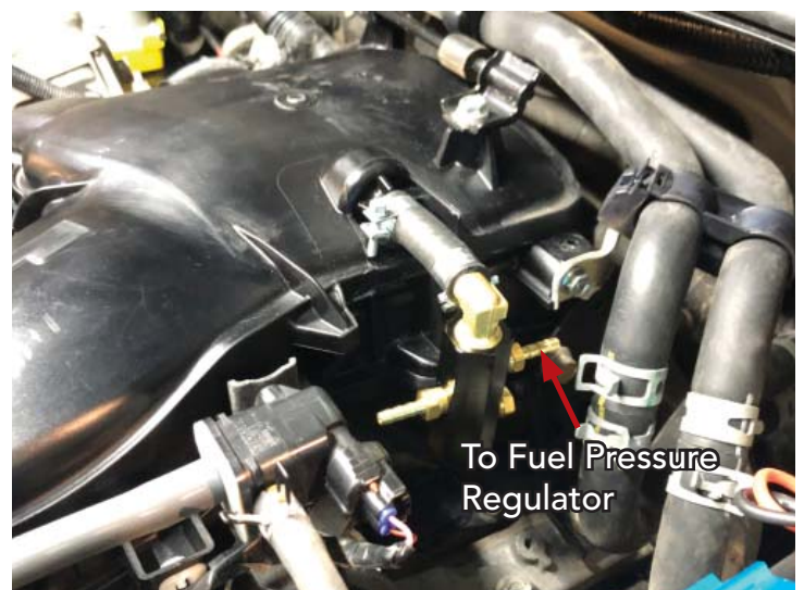
Vacuum Manifold Installed
