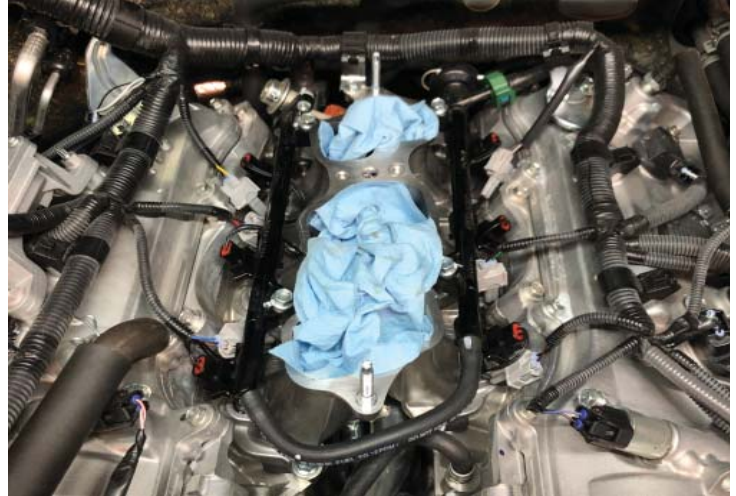
Injectors Installed With Adaptors
