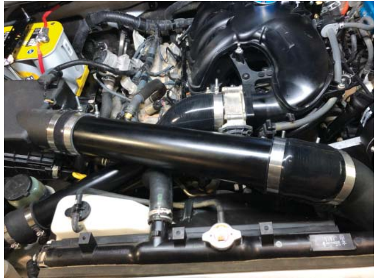
Air Inlet Tube Installed
