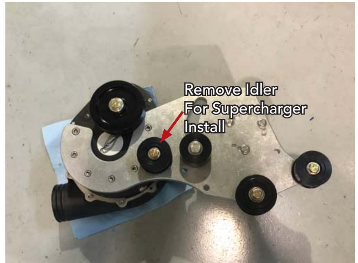
Supercharger Installed Onto Bracket
