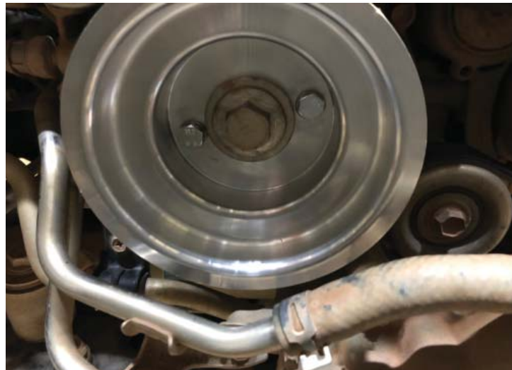
Crank Pulley Installed
