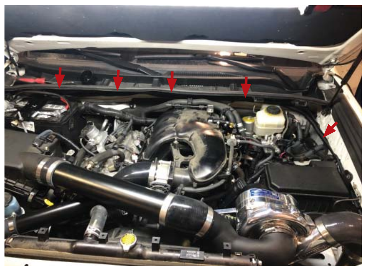
Battery Cables Routed
