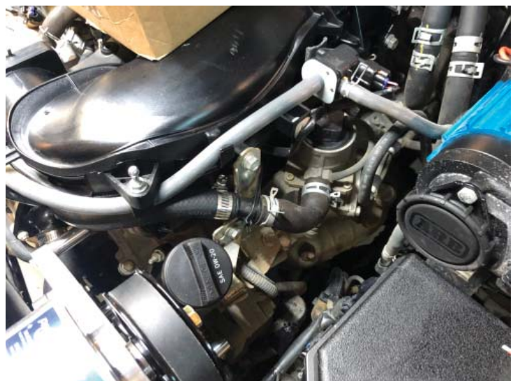
Drivers Side Air Pump Connection
