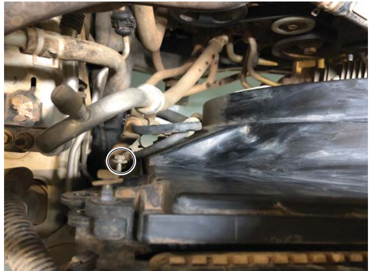
Transmission Cooler Line Bolt
