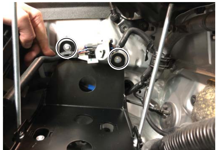
Battery Tray Side Bolts
