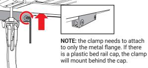
Fold the cover closed. Install the bed flange extender clamp (J) as shown. The clamp will slide onto the metal edge of the truck bed rail and align with the rear cover clamp. With the clamp positioned, hand-tighten the screws with the 5/32" hex key wrench (L). Swing the clamp down so that the jaw is under the edge of the bed flange extender. Push the clamp handle toward the bed wall to lock it in place. Repeat on the opposite side of the bed.
