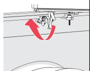
Slide the tether clamp onto the metal end of the truck bed flange and tighten the knob.
