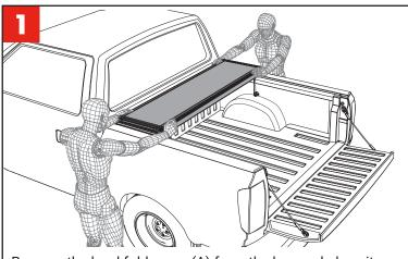
Remove the hard fold cover (A) from the box and place it on the cab end of the truck.
