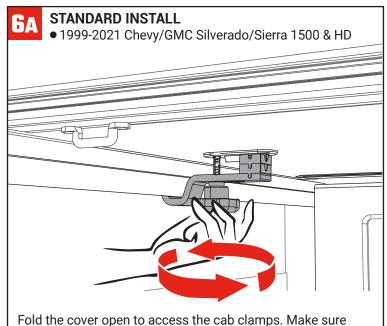
that the cab clamp is under the metal bed flange of the truck bed rail. Hand-tighten the knob. Repeat on the opposite side of the truck bed.
