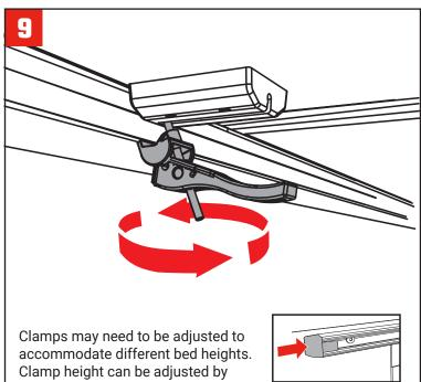
turning the clamps clockwise or counter-clockwise to move the clamp higher or lower as needed.
