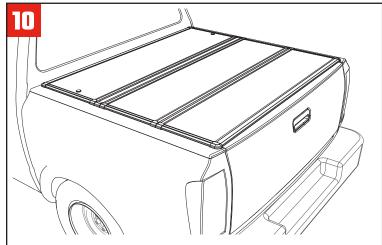
Close tailgate to check how the cover fits and adjust as needed. To make changes, loosen the cab clamps (E) and shift the cover into the appropriate spot, then retighten the cab clamps.
