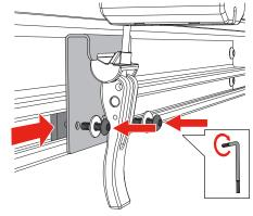
Fully close the cover. Insert the slide plate (M) into the end of the factory cargo rail, align the clamp bracket (N) with the tail clamp. Attach the clamp bracket (N) to the slide plate (M) using the screws (O) and washers (P), tighten the screws (O) with the T27 Torx wrench (Q). Swing the tail clamp down to lock it to the clamp bracket (N). Repeat the steps on both sides of the bed.
