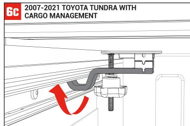
Lay the cab panel back down and fold the entire cover back up as shown in Step 1 to access the cab clamps (E). Hook the cab clamp (E) directly under the edge of the factory cargo rail. Tighten the lock knob (H). Repeat the steps on both sides of the bed. **Snug firmly but do NOT overtighten.** Reinsert any tie-down cleats in desired positions.
