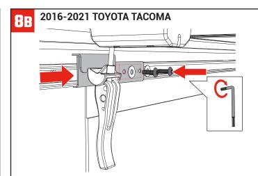
Fully close the cover. Slide the slide plate (M) into the end of the factory cargo rail, align the clamp bracket (N) with the tail clamp. Attach the rear clamp brackets (R & S) to the slide plate (M) using the screws (O) and washers (P), tighten the screws (O) with the T27 Torx wrench (Q). Swing the tail clamp down to lock it to the clamp bracket (N). Repeat the steps on both sides of the bed.
