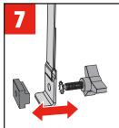
The tether hardware comes assembled on the tether (I). Unscrew the knob (L) from the slide block (J) and separate the block, knob and washer (K).
