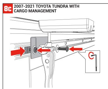
Fully close the cover. Slide the slide plate (M) into the end of the factory cargo rail, align the clamp bracket (N) with the tail clamp. Attach the clamp bracket (N) to the slide plate (M) using the screws (0) and washers (P), tighten the screws (0) with the T27 Torx wrench (Q). Swing the tail clamp down to lock it to the clamp bracket (N). Repeat the steps on both sides of the bed.
