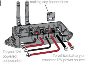
\*Suggested gauge of wire for direct connection: 10 AWG **REMARK:** For wire gauge under 10 AWG a terminal block connection is recommended.
