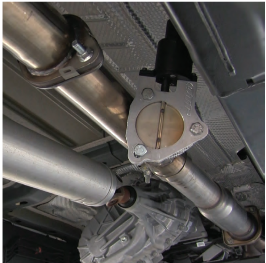
Image C: QTEC Valved installed on Aggressor Pipe
