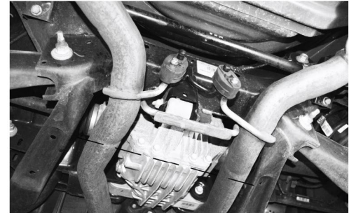
Use seam between diff cover and diff housing as cut line
